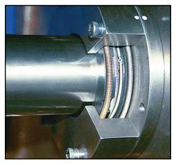
RTV gas-sealing wiper
