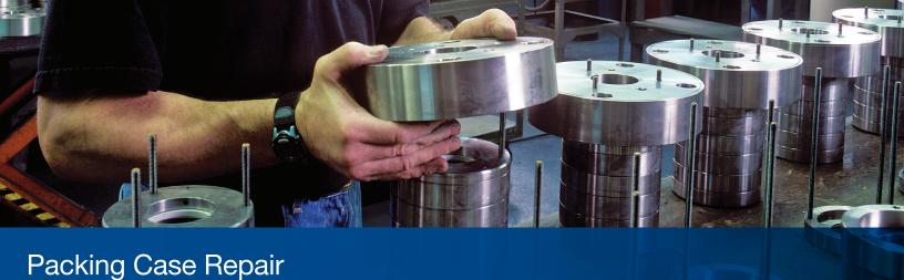
Worn rod packing is a major source of inefficiency and gas losses in reciprocating compressors. Cook Compression<sup>®</sup> repairs all types of packing cases and sealing components, helping operators improve profitability and reduce fugitive emissions.
