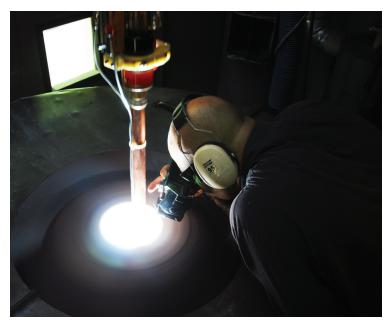
PlasKote50+<sup>®</sup> plasma coating reconditions cylinder bores without using liners
