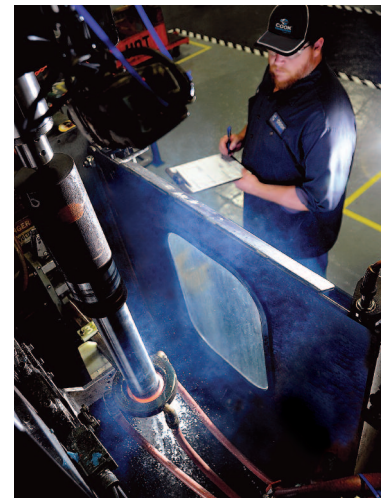
Induction hardening a piston rod at the Cook Compression Service Center in Odessa, TX.
