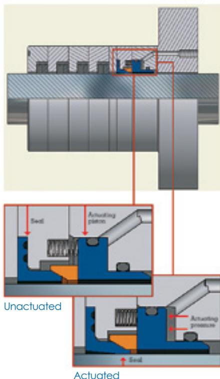
Any combination of manual or automatic interlocks may be used to activate the seal. When activating pressure is released during compressor start-up, the Static-Pac seal lifts off the rod surface to allow free movement of the rod.
