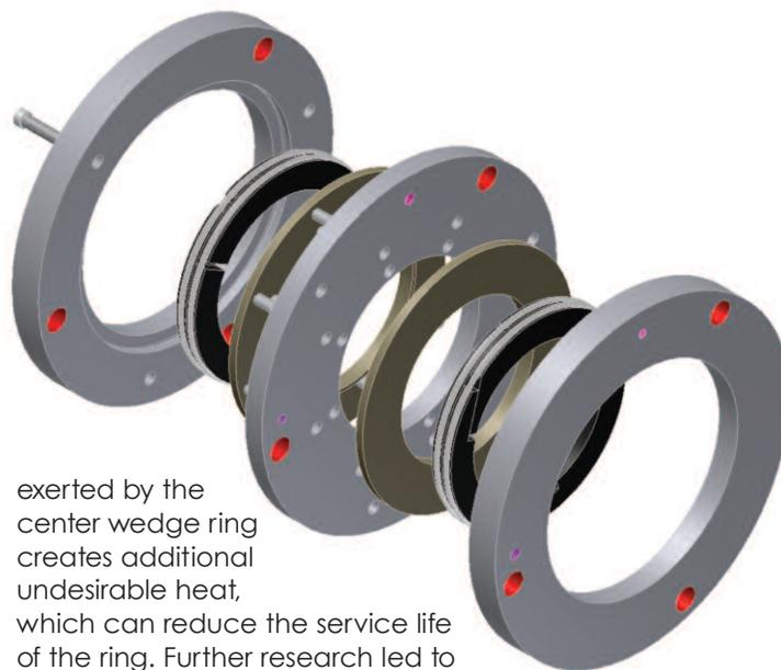
exerted by the center wedge ring creates additional undesirable heat, which can reduce the service life of the ring. Further research led to the development of Low-Friction (LF) technology, which creates effective side-loading without using a wedge ring.
