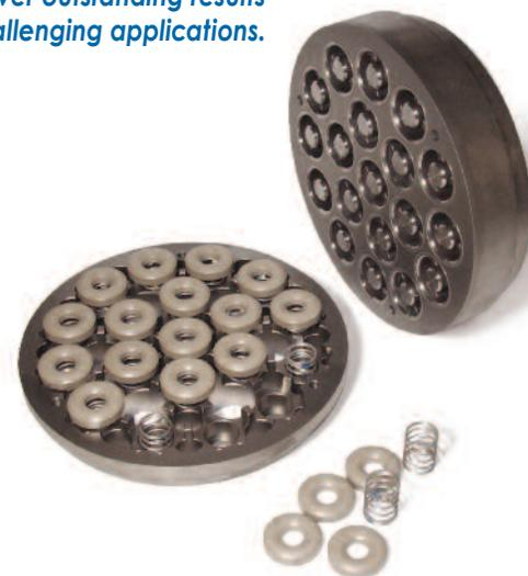
available in diameters ranging from 2.0 inches (50.0 mm) and up, and can be used in any model compressor where the valve envelope is sufficient to accept the design. They have been used in a wide variety of services and operating conditions, including pressures from 0 to 5,000 psi (0 to 350 bar) and with gases ranging from hydrogen and ethylene to flare and natural gas.
