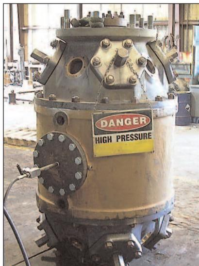
Compressor cylinder being hydrostatic tested at 1½ the maximum working pressure
