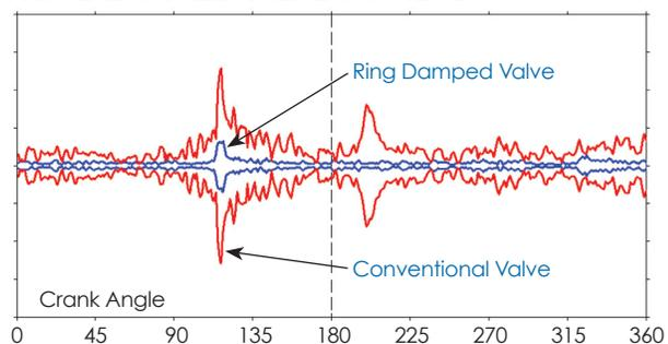
*Accelerometer trace from valve cap shows significantly lower impacts of Ring Damped Valve vs. conventional valve*
