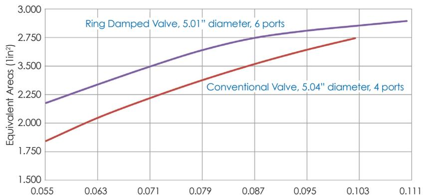
*Ring Damped Valves operate at higher lifts, increasing flow and saving energy*
