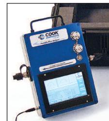
Sentrix portable thermal mass flow meter
